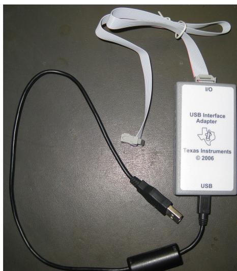
Figure 3. Picture of USB-TO-GPIO
