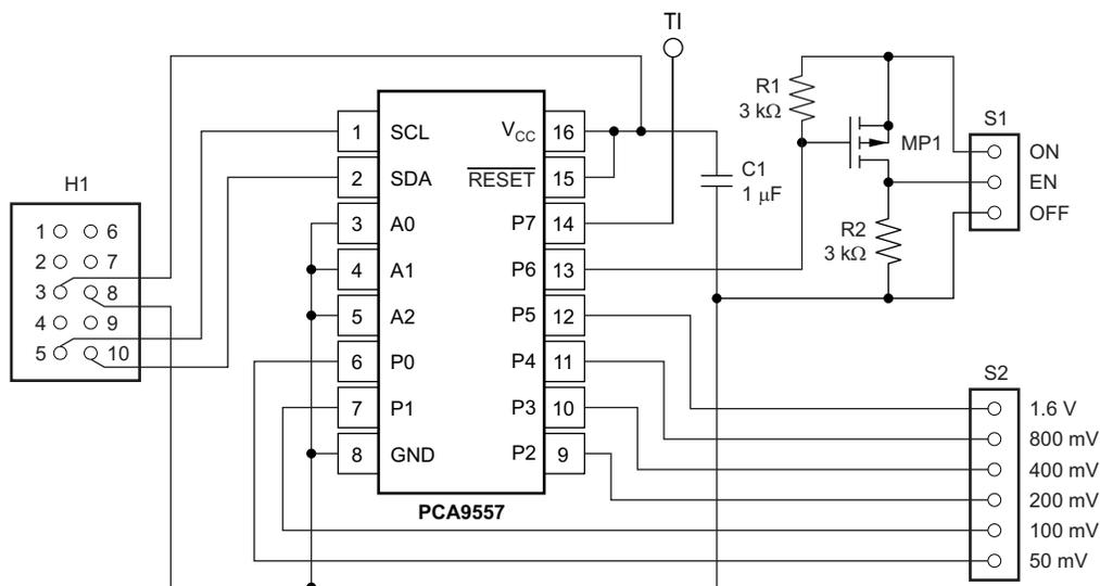
**Figure 1. Schematic of I<sup>2</sup>C IO Expander Board**
